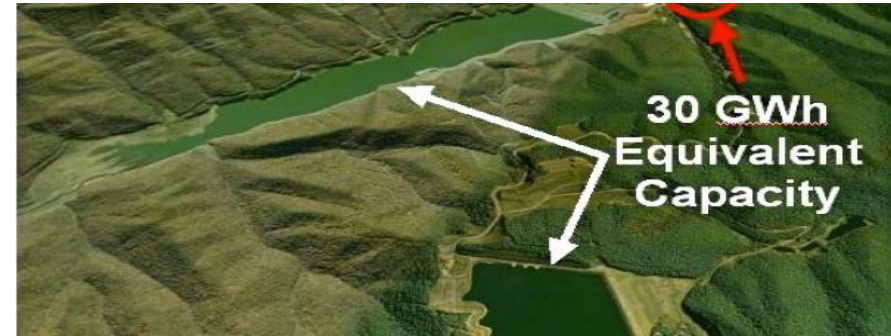
Bath County Virginia, USA 3,030 MW pumped storage “world’s biggest battery”
