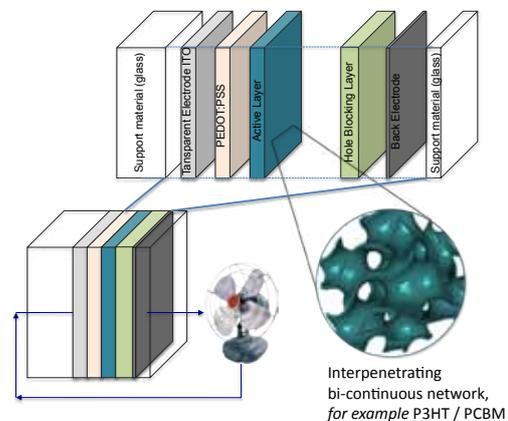
Above: Bulk Heterojunction Solar Cell (BHJ)
