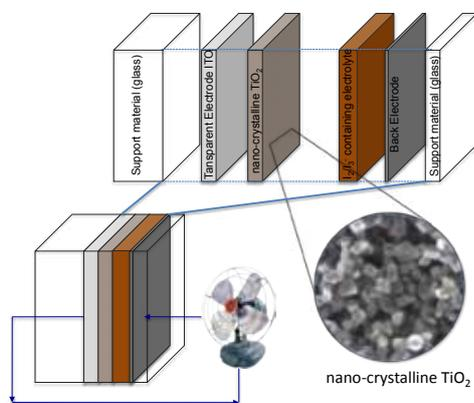
Above: Dye Sensitised Solar Cell (DSC)
