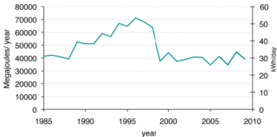
Figure 40. Gas usage in our house, before and after the heating system was replaced. The gas use started to climb from around 1988 and then dropped abruptly in 1999.
