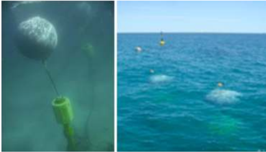
Figure 12. Buoys used for an ocean powered combined desalination and electric power generation plant. From Carnegie website.
