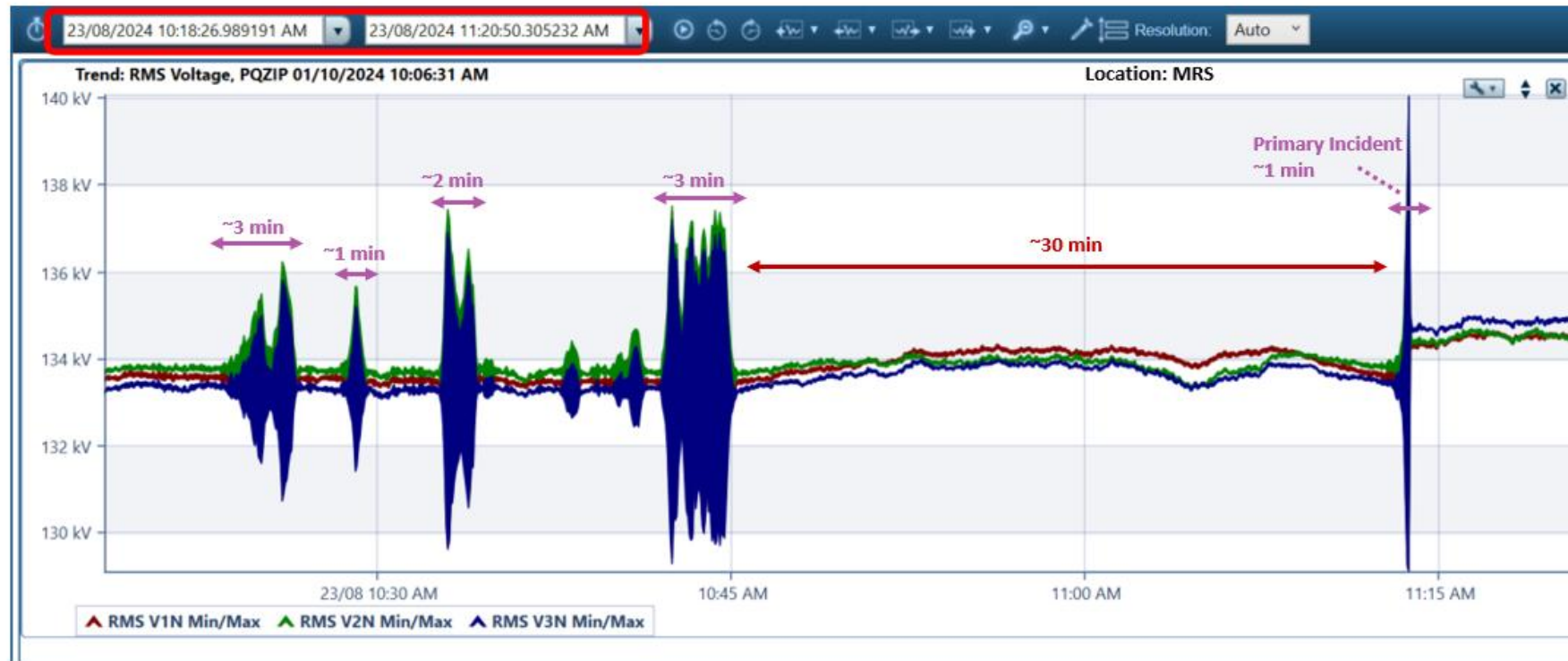
Multiple voltage oscillations in EC on 23-08-2024
