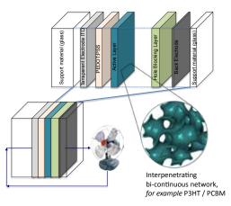
Above: Bulk Heterojunction Solar Cell (BHJ)
