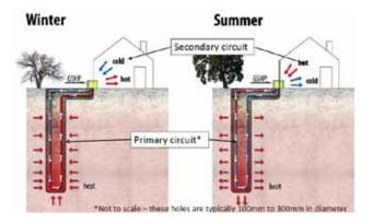
Imagine trying to dump heat from your house into air at 40°C, when you could be using 18°C ground. Unlike many other sources of renewable energy, GSHP systems can potentially be used in almost any geographic location and the energy is available 24/7 – rain, hail, sun, storm or calm. This gives GSHP systems a significant advantage over alternative forms of renewable energy.
