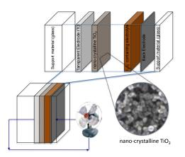
Above: Dye Sensitised Solar Cell (DSC)
