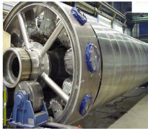
Coilwound Heat Exchanger
